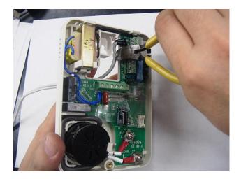
③Let cable clamp through the upper part of the hole to pull out cable and fasten the cable clamp halfway.
